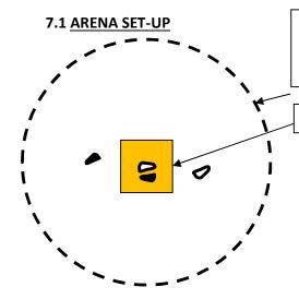
RING (4.0 m DIA) in middle of 8m by 8m rubber mat of 40 mm thick.
